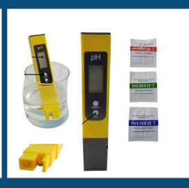
Used for measuring the acidity or alkalinity (pH) of a liquid.
