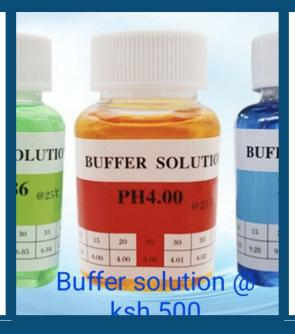
Used for calibrating pH meters to ensure accurate acidity or alkalinity measurements.
